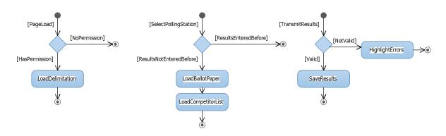
Figure 2: Activity Diagrams for Page Load, Polling Station Select and Transmit Results
