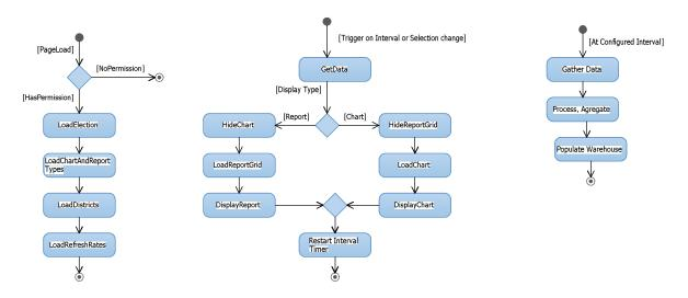
Figure 8: Activity Diagrams for Page Load, Report Triggers and Updating Warehouse
